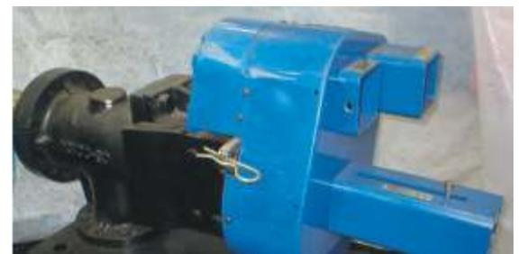
**Slurry actuator device with standard safety guarding fitted**
