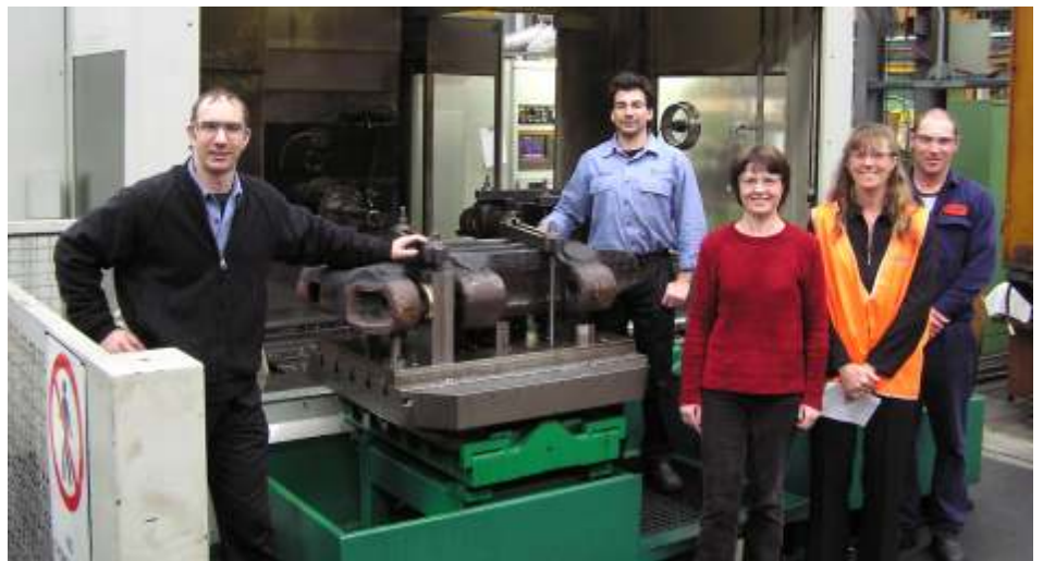
One of the machining centres installed to manufacture track pads for Hitachi with some of the Hofmann team who are involved with the manufacture of track pads.
