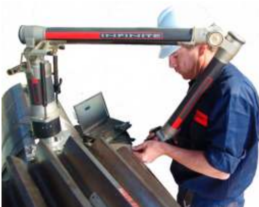
A mill pinion in the middle of the Atacama Desert in Chile being accurately measured.
