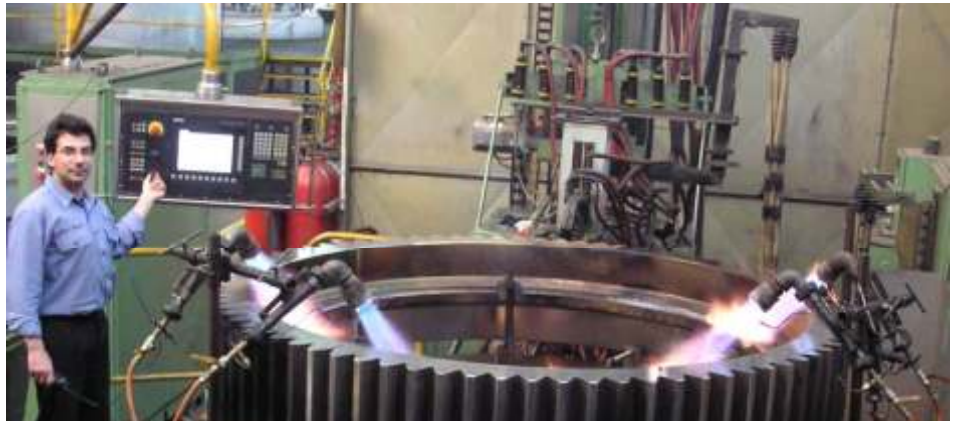
A Bucyrus 495 shovel crowd gear undergoing tooth by tooth full contour induction hardening on our CNC controlled induction hardener.
