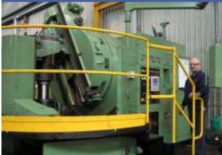
Bucyrus dragline motor pinions being hard cut on Our CNC Maag Gear Planer.
