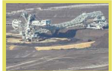
View of a typical bucket wheel reclaimer. The gearbox will be installed on the bucket wheel. Note: This gear box both supports and drives the bucket.
