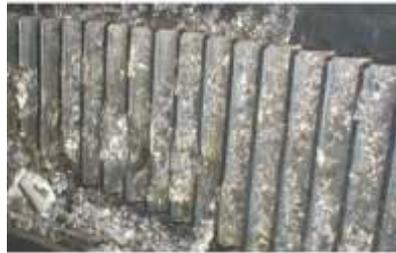
**Minimal damage to Hofmann Induction Hardened internal ring gear. Considering the rest of the case hardened gears and bearing were completely destroyed it is surprising that the induction hardened ring gear teeth are intact.**
