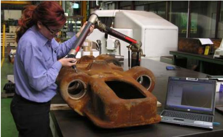
**In a move that will drastically reduce the time spent on measuring complex components requiring re-engineering, Hofmann has acquired a fully portable co-ordinate measurement machine.**
