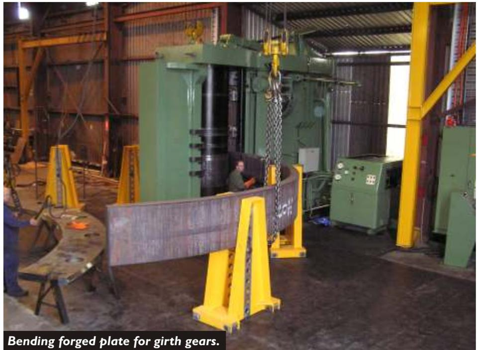
Bending forged plate for girth gears.
