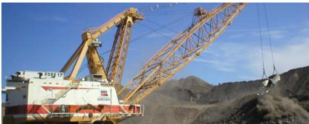
UDD hoist and drag arrangement, utilising the unique hoist drum and latest in gear technology.
