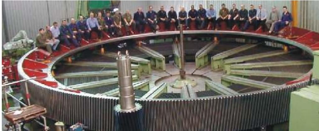
*This 12-metre diameter girth gear is shown during manufacture in our Bassendean plant. Hofmann Engineering is able to manufacture Forged Fabricated and Forged Fabricated Induction Hardened girth gears to 15m in diameter. We can also offer SG Iron, Cast Steel and Austempered SG Iron alternatives.*
