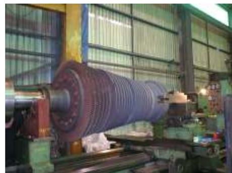
**Rotor repair under way in our plant**
