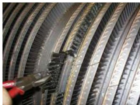
need of a blade changeout. This involved removal of the damaged blades by machining, and installing and machining new blades required to get the turbine back into operation.
