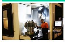
capability allows the table to rotate up to a speed of 800rpm, Hofmann Engineering can produce for the future. with an electric motor actuated table producing 36 kW of power.
