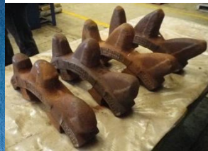
From Left To Right: Sizer teeth at different stages of wear for analysis, Wear profiling of sizer tooth, Metallurgical laboratory inspection equipment, micrograph of a trialled hard facing consumable with a hypereutectic structure of primary carbides designed for extreme abrasive wear.
