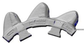
From Left To Right: Sizer teeth at different stages of wear for analysis, Wear profiling of sizer tooth, Metallurgical laboratory inspection equipment, micrograph of a trialled hard facing consumable with a hypereutectic structure of primary carbides designed for extreme abrasive wear.
