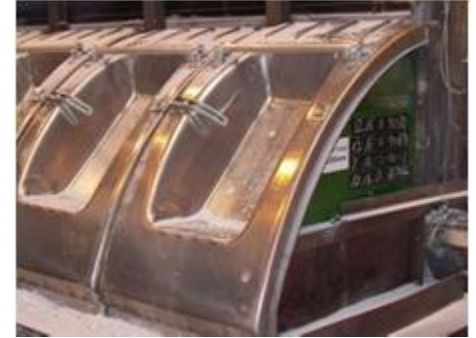
ABOVE: SMELTER POT DOOR COVERS WITH HINGES AND LATCHES WELDED ON
