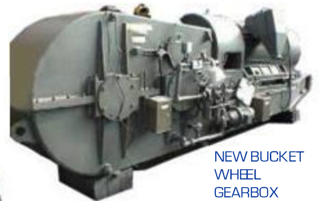
Hofmann Manufactured new Bucket Wheel Gear box (630kW) complete with torque arm (see over for further details).
