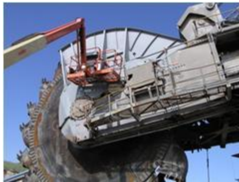
The Bucket Wheel and fully enclosed Bucket Wheel Gear box situated at the end of the boom.
