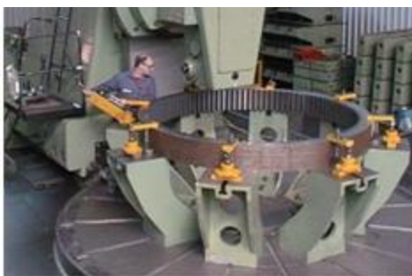
Slew Bearings - Induction hardened and precision ground..
