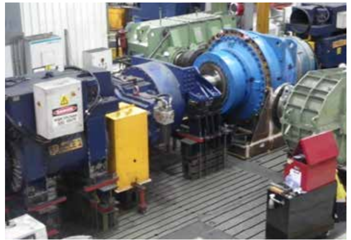
Above: Hofmann refurbished P2SA-38 (2800kW) HPGR Gearbox under load test.
