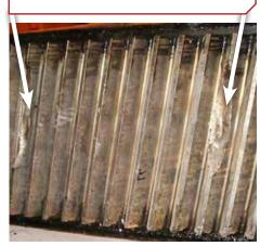
Forged steel fabricated girth gears overcome cast steel cracking problems. Forged steel gives the highest crack and impact resistance.
